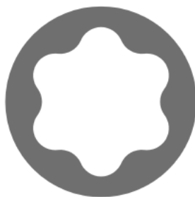
Shape of ASA screw head
